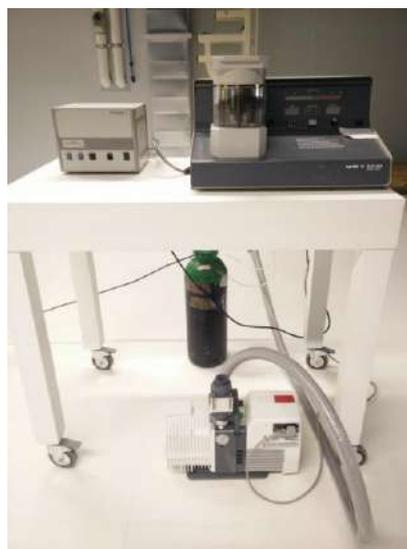
Figura 27: Imagen del Sputter coater (modelo SCD 005, fabricante BAL-TEC).
