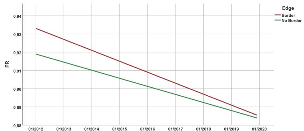
Figure 7. Variation of the PR for a PV production unit located or not placed at the edge per elapsed month. Own elaboration.
