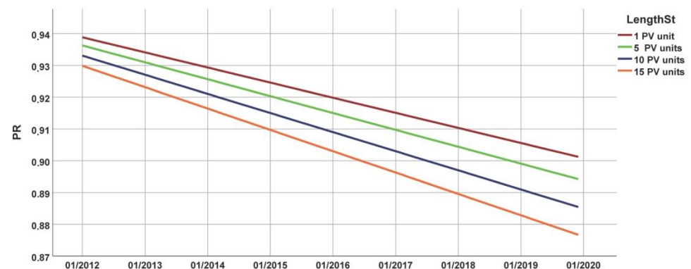
Figure 8. Variation of the PR for PV production units in streets that have 1 to 15 units per elapsed month. Own elaboration.
